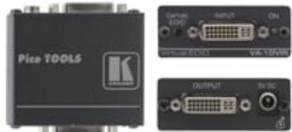
The VA-1DVIN is an EDID emulator for DVI-D signals. The unit can capture an EDID setting in non-volatile memory from the output allowing convenient and reliable connection to the source
